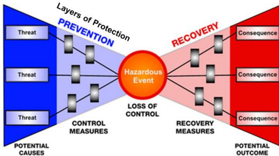
Figure 1: Schematic of BowTie Safety Assessment Process
